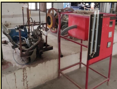
Multi fuel computerized control Single cylinder VCR engine test rig
