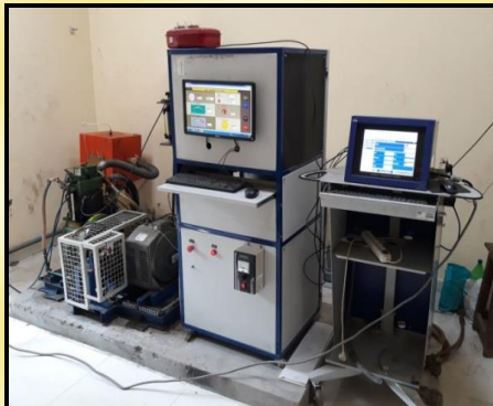
Multi fuel computerized control Single cylinder VCR engine test rig
