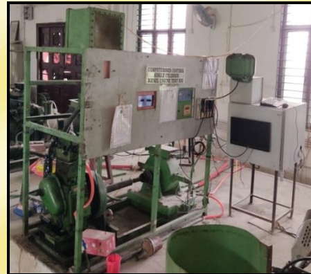
Computerized control Single cylinder four stroke Diesel engine control test rig
