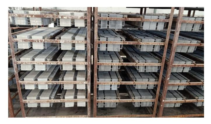
Dark one plate is for Cathode and bright one is cathode. After this plates cut into 3 pieces. After this plates placed into batteries in acid and charging process is done. After complete process of their 1 plant we then had little snacks and beverages. Their hospitality s very good.
