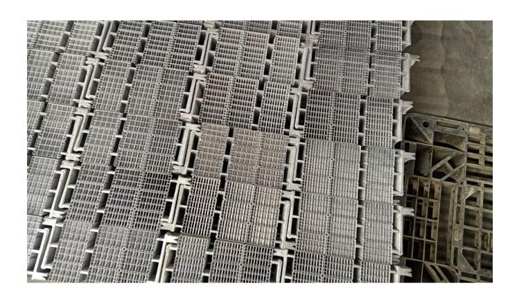
After this pasting process is started in pasting process paste of lead oxide and sulfuric acid is pasted on grid of lead. After this process amount of lead is nearly 70% present.
