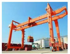
At Adani Port, we encountered RMG (rail-mounted gantry) cranes, pivotal in the container handling process encompassing loading, unloading, and stacking operations. These robust machines, integral not only to the port but also to container terminals and railway transfer yards, epitomize efficiency in cargo management. Noteworthy were the varying capacities observed, ranging from 60 to 80 tons, underscoring the versatility of these
